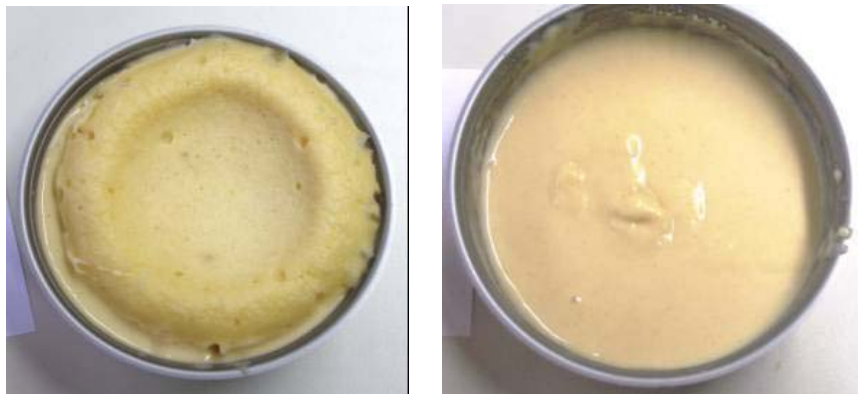
Figure 6.14: Solidification of egg batter in Ø 127 metal container after 186 s in the Micromax oven.
