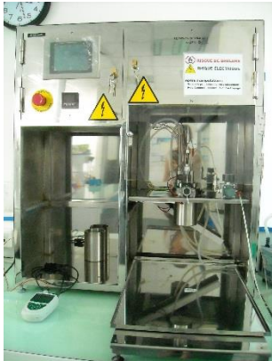
Thermoresistometer Mastia® - Device to measure vitamin C degradation at high temperature
