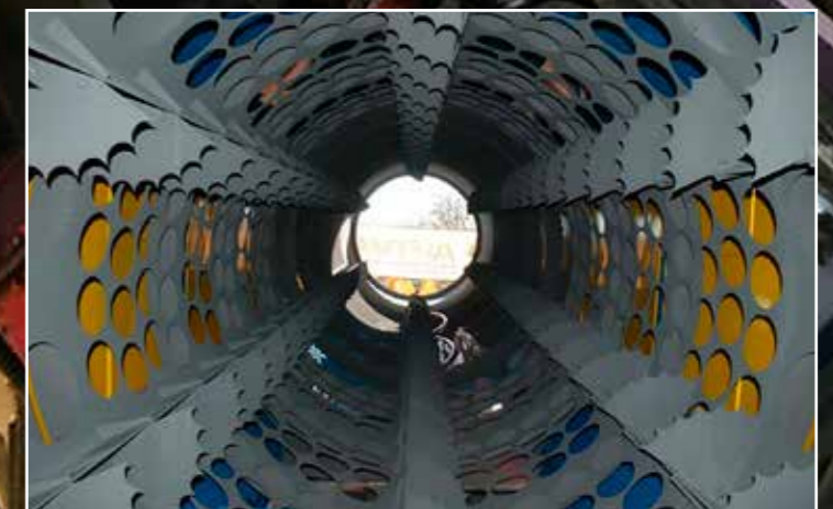
▲ Trommels (above) are used to separate different waste flows in materials recycling facilities. Small sized items fall through the holes of the trommel.
