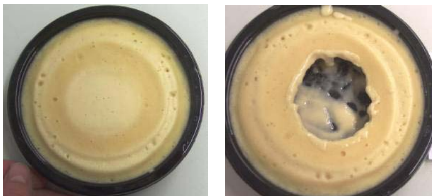
Figure 6.15: Solidification of egg batter in Ø 127* plastic container after 60 s in the Panasonic oven.
