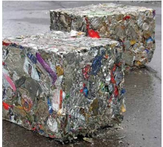
Figure 10: Grade 6E- Clean Steel Cans- bundles, BMRA UK specifications for metals recycling.
