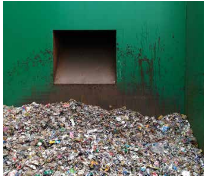
Figure 9: Left, steel packaging scrap coming out of a second sorting step. Right, impurities. ©APEAL
