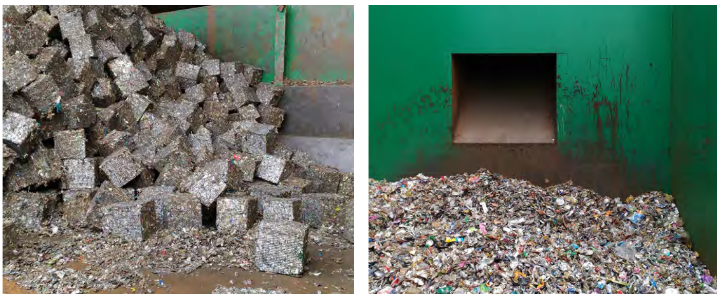
Figure 12: Left, steel packaging scrap coming out of a second sorting step. Right, impurities. ©APEAL
