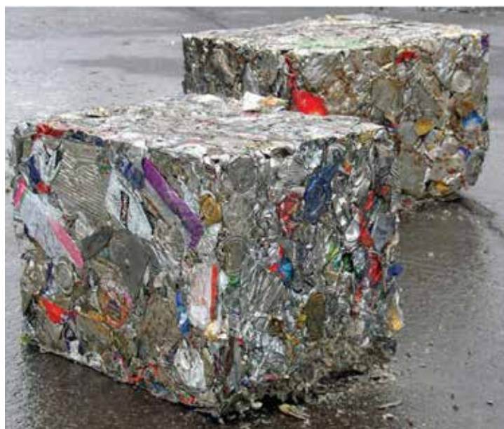
Figure 9: Grade 6E- Clean Steel Cans- bundles, BMRA UK specifications for metals recycling.
